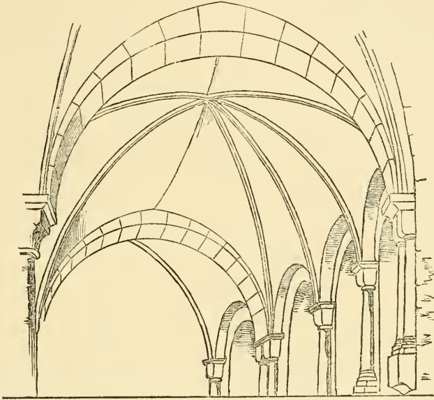
Fig. 84.—Showing the development of the cross-ribbed arches, and distribution of the pressure.
