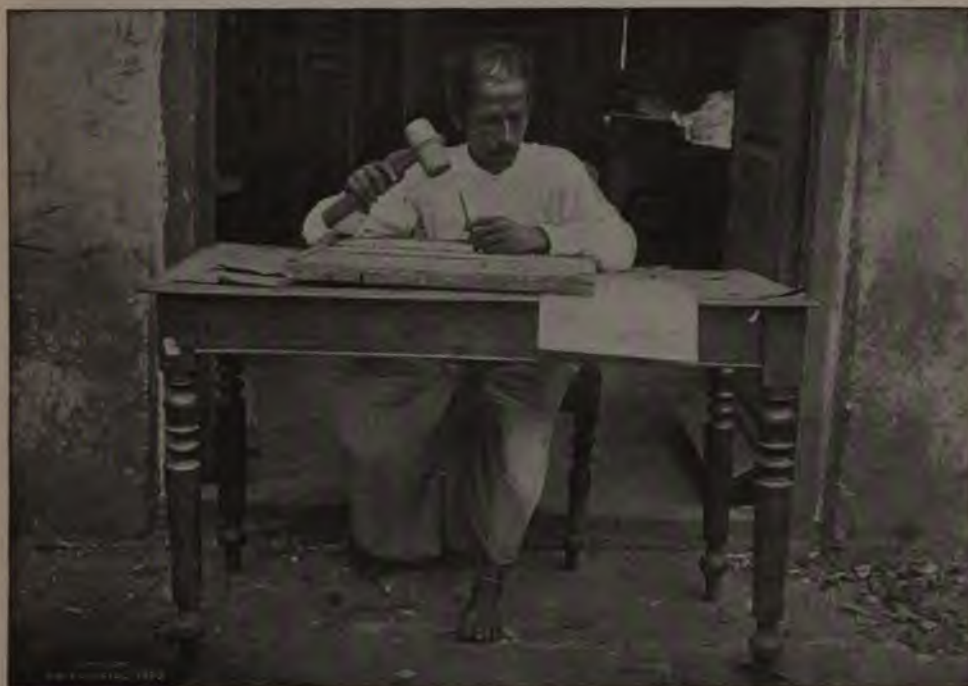
MAKING DIES USED FOR PRINTING BOOKS FOR THE BLIND.
